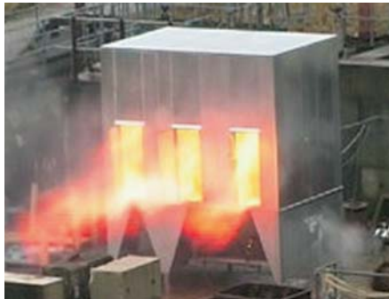
Full scale explosion test of NF2000
